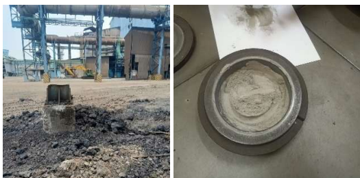
Fig. 1. Pretreatment of steel slag: (A) Slag collection from the field, (B) Particle size reduction by crushing and grinding.
