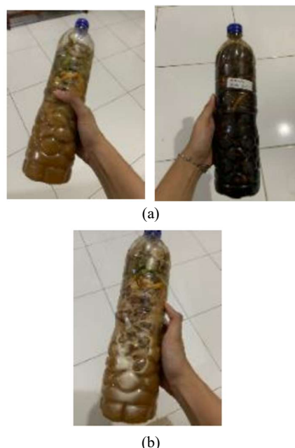
Fig. 3. Visual observation of the biopesticide fermentation process: (a) Comparison of the final liquid characteristics between Formulation A and Formulation B on day 7, and (b) Active fermentation phase indicated by foam formation in Formulation A on day 5.
